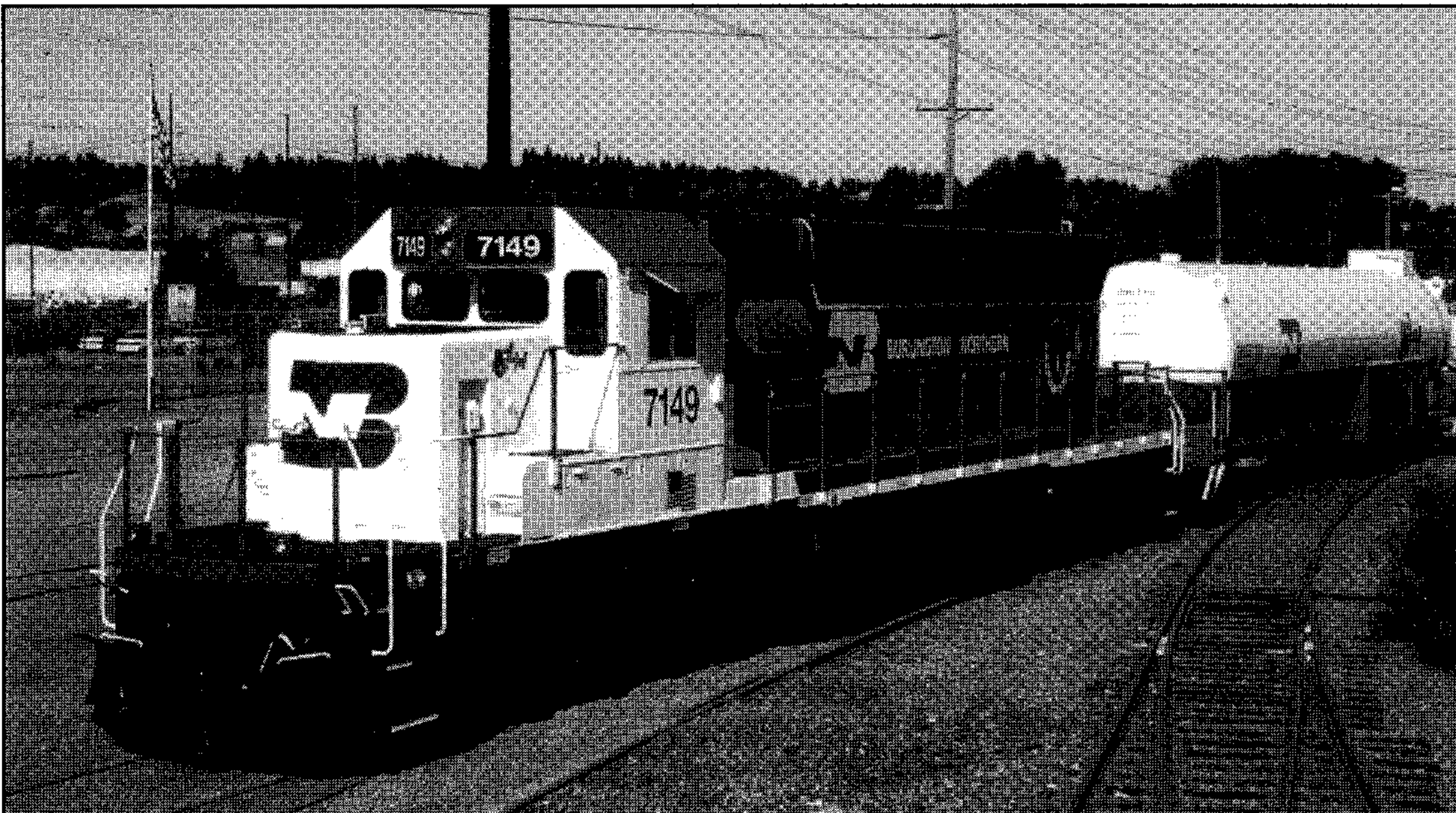
Burlington Northern installed the ECI dual-fuel conversion in this SD-402-2 locomotive powered by a 16-cylinder EMD Model 645 E3B engine. The tender car behind it carries enough LNG to fuel a pair of these engines for a range of 1,600 miles.
